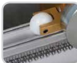
Machine-Application results in a uniform, flat splice – even on belts prone to belt wave
