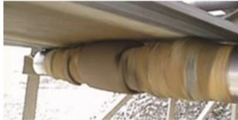
Carryback material buildup on a steel roller
